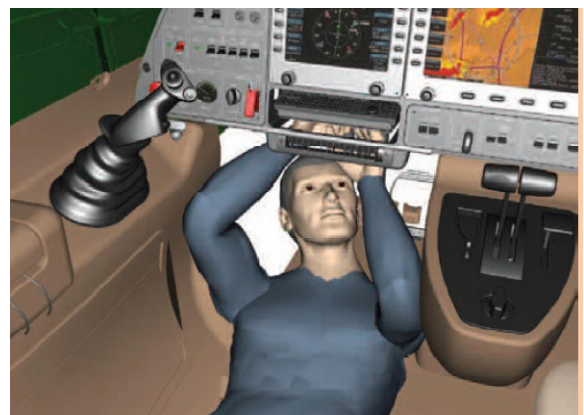
Figure 8: Tecnomatix simulation of a repair in an airplane cockpit (Siemens).
